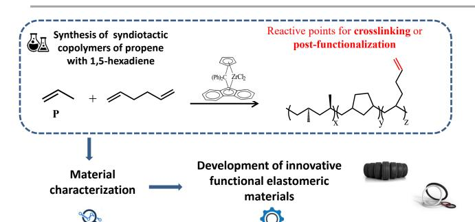
Innovative functional elastomers based on syndiotactic homo and copolymers
